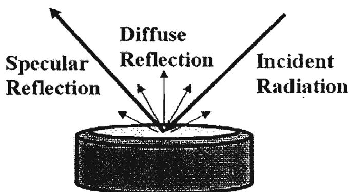
**Figure 2.6:** Schematic diagram showing the diffuse reflection.
