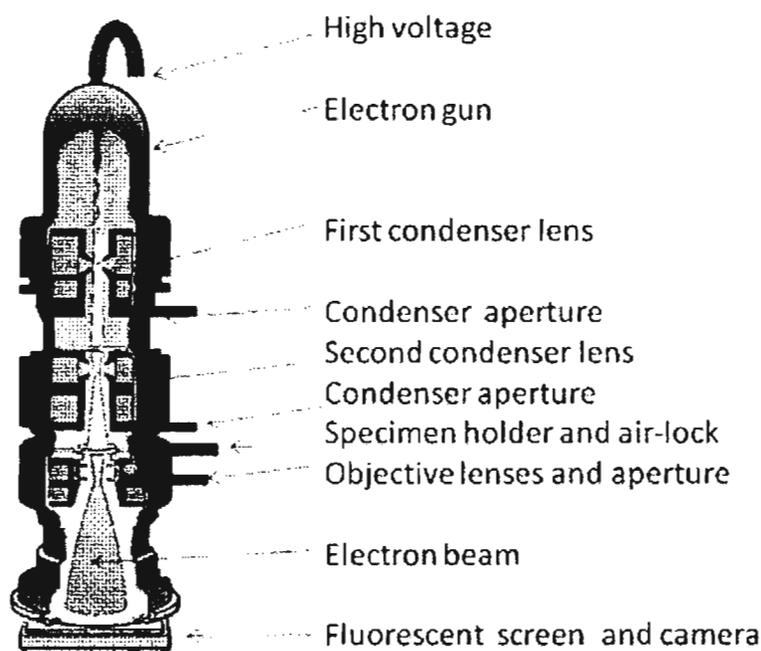
**Figure 2.3:** Schematic diagram of TEM
