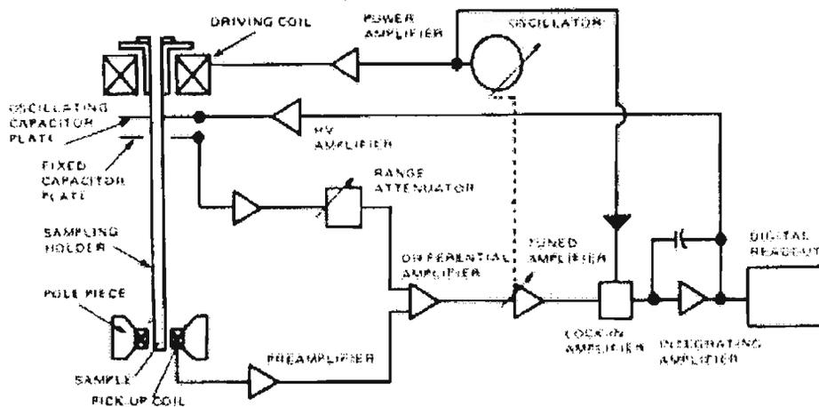
**Figure.2.7:** Block diagram of vibrating sample magnetometer.
