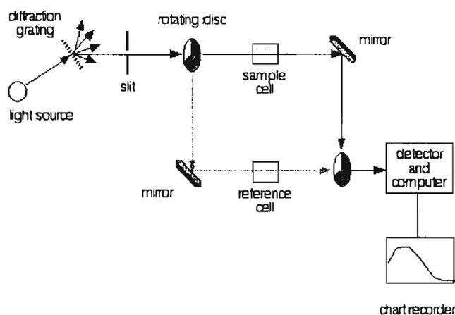
**Figure.2.5:** Double beam UV-visible spectrometer
