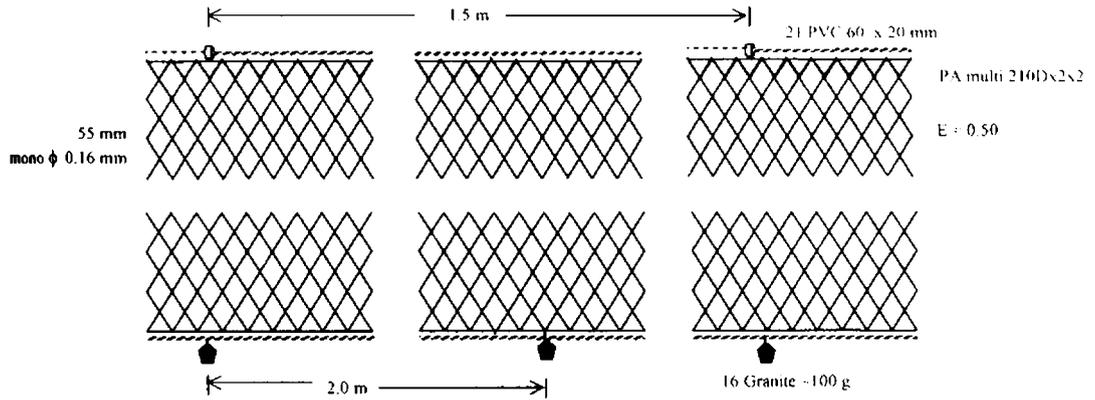
**Fig. 41. Experimental gillnet for mesh selectivity studies with 55 mm meshes**
