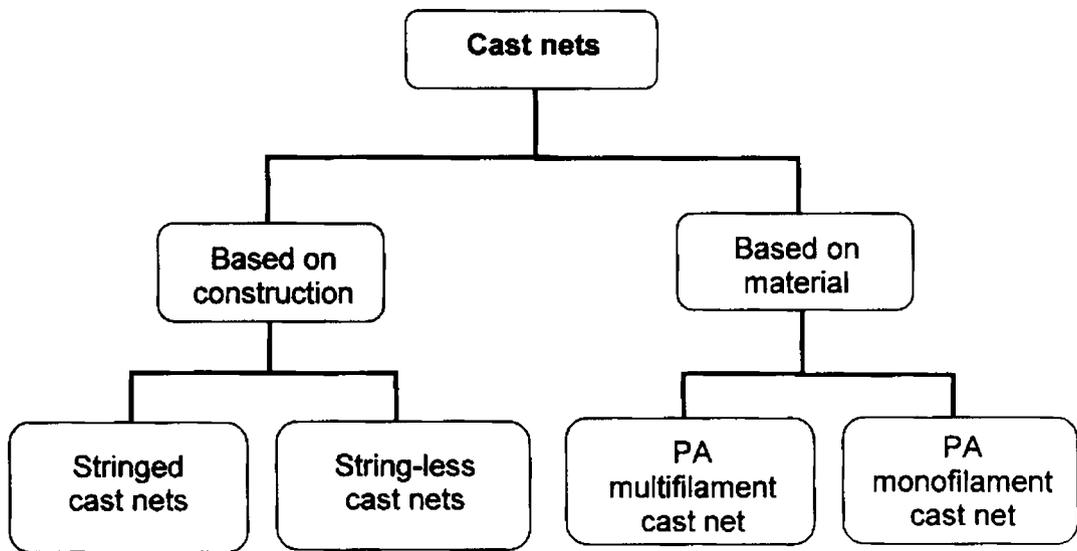
**Fig. 90. Classification of cast nets**
