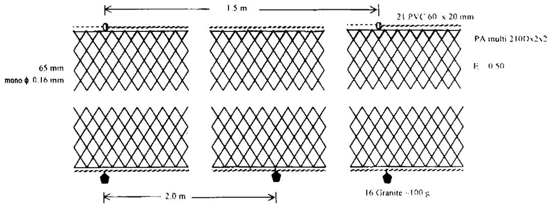
**Fig. 42. Experimental gillnet for mesh selectivity studies with 65 mm meshes**
