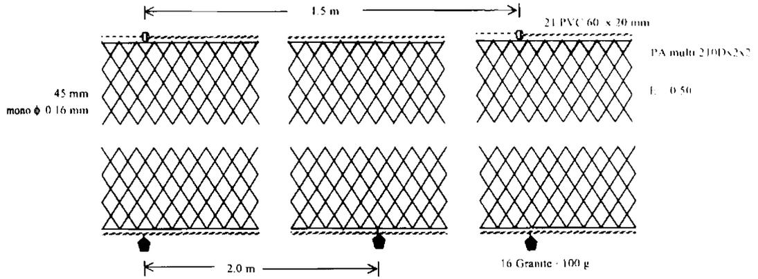
**Fig. 40. Experimental gillnet for mesh selectivity studies with 45 mm meshes**
