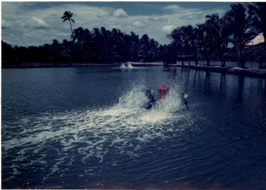
B – Paddle wheel aerated semi-intensive farming at Mundapuram
