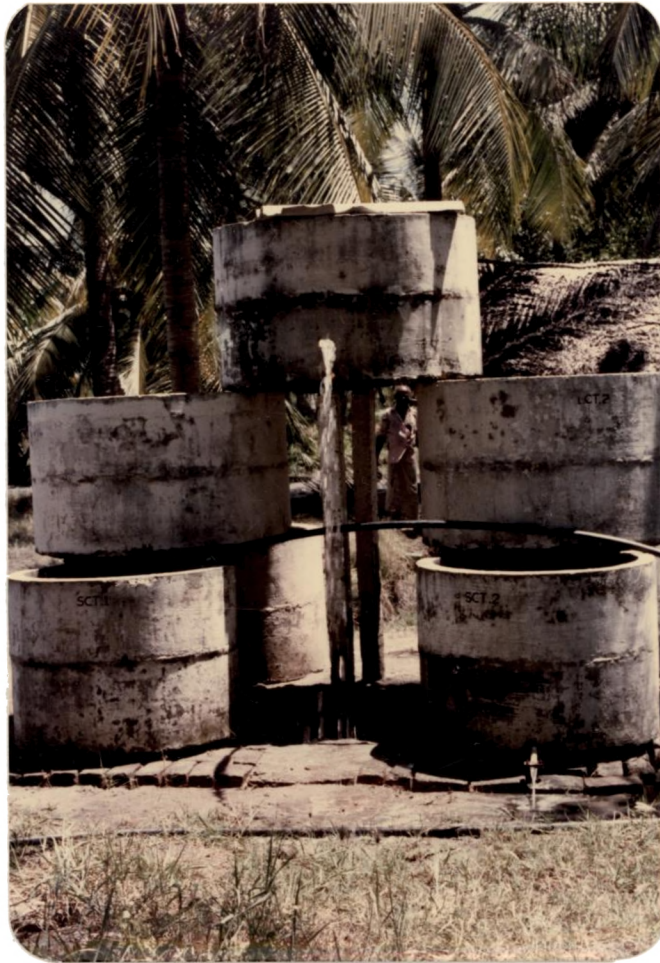
A - Circular cement tanks set-ready
