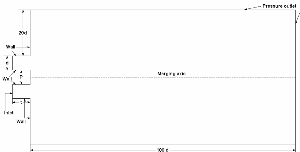
Fig 6.7 Solution domain and boundary types of twin jet
