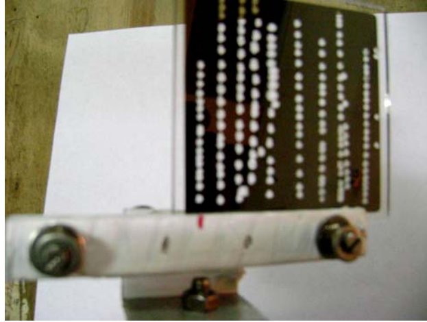
Figure 2.1 Photograph of the target plate fixed on a holder. Each circular spot represents the ablated areas.
