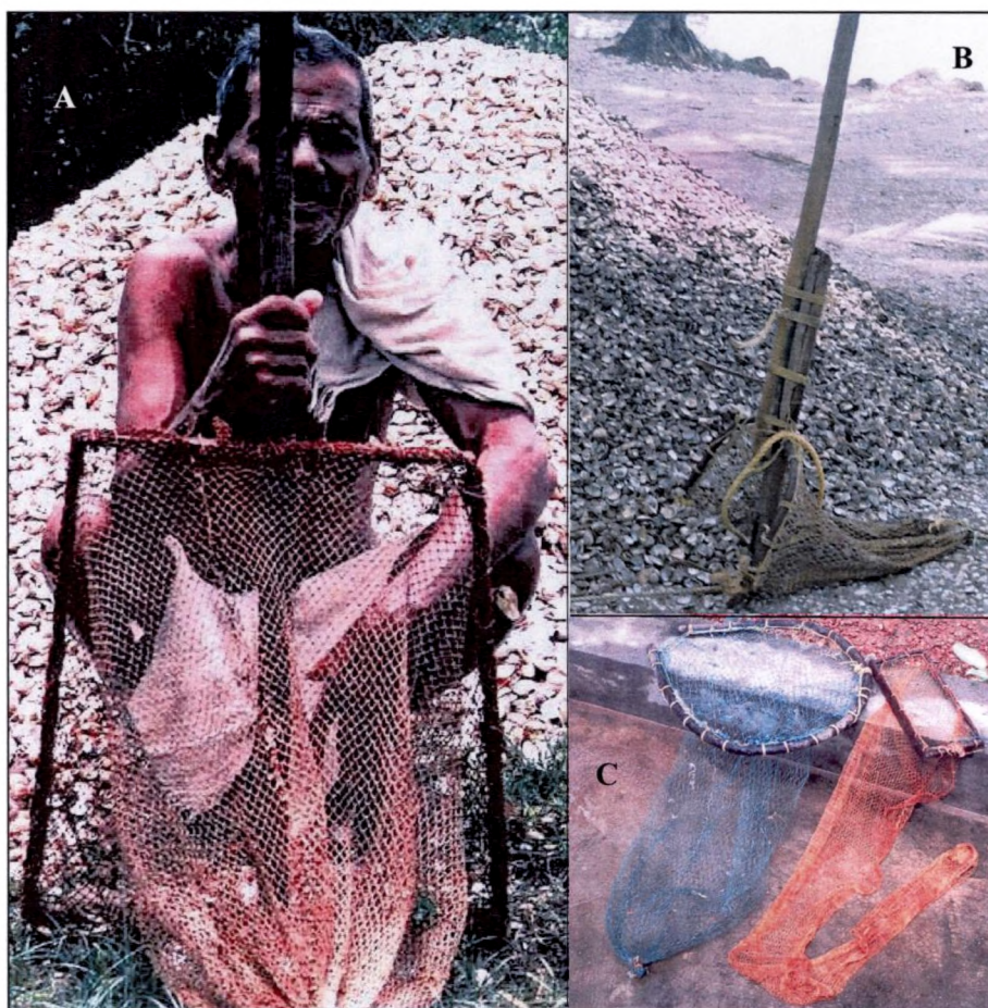
A-Stick held scoop net B-Hand operated dredge C- Nylon and Polyethylene Scoop nets
