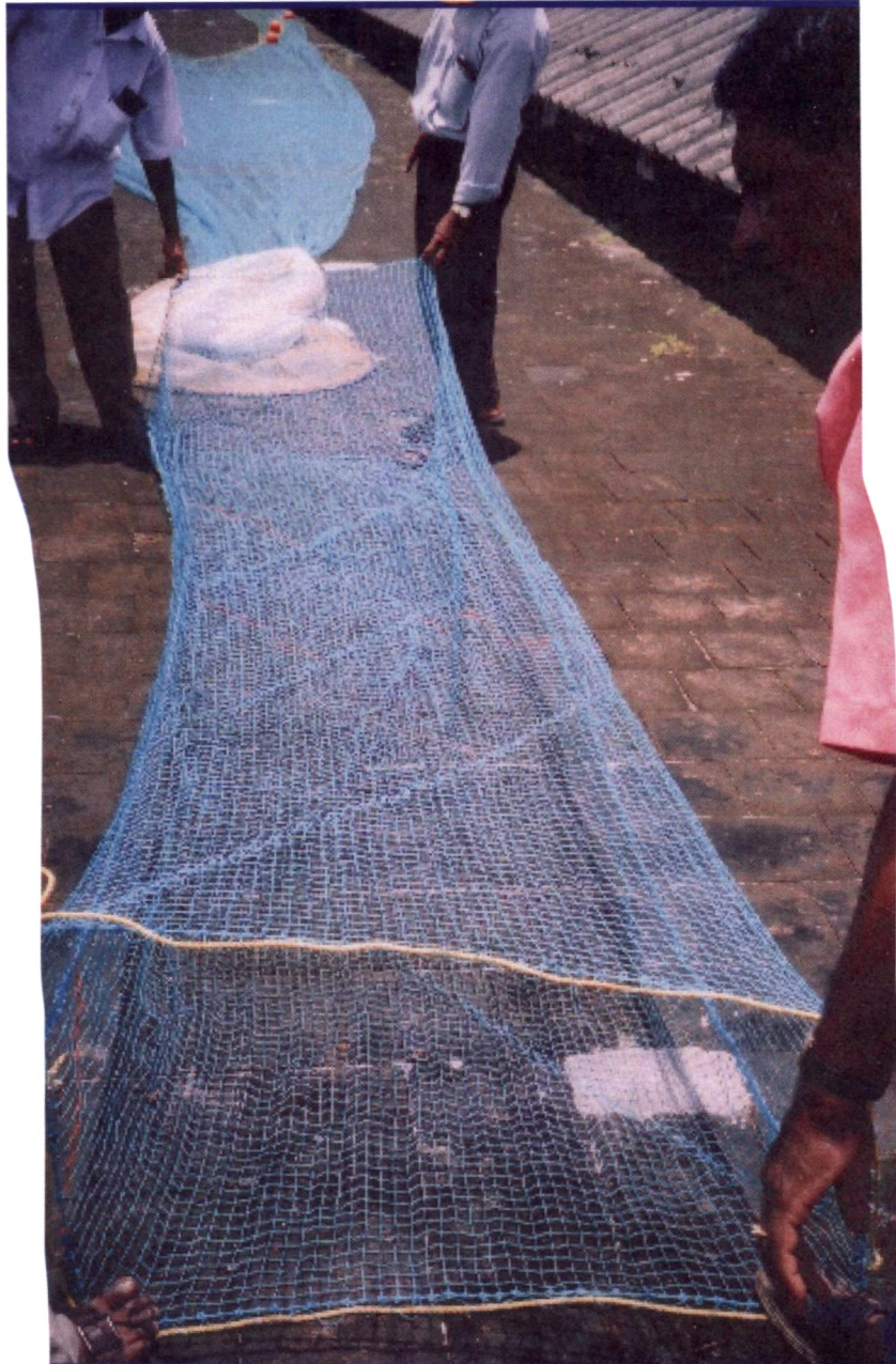
Fig 50: A view of square mesh codend
