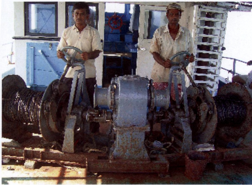
Fig 13: Releasing of warp line
