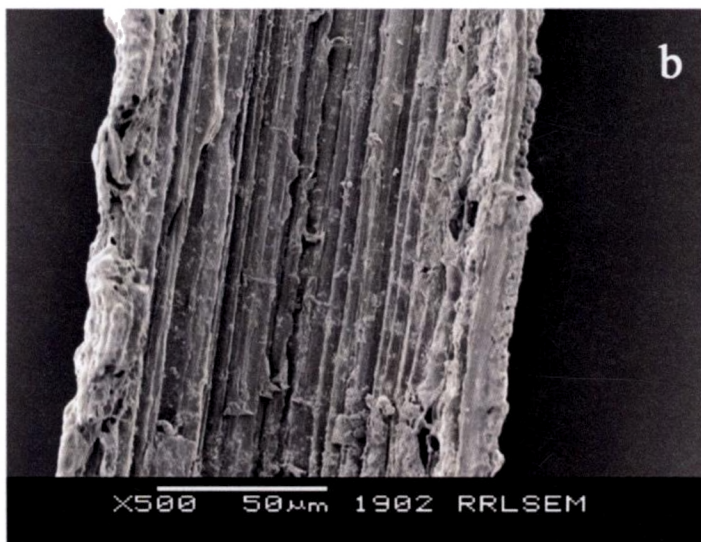
(b) Appearance of rice straw after 48 h of fermentation with S. psammoticus under solid-state culture
