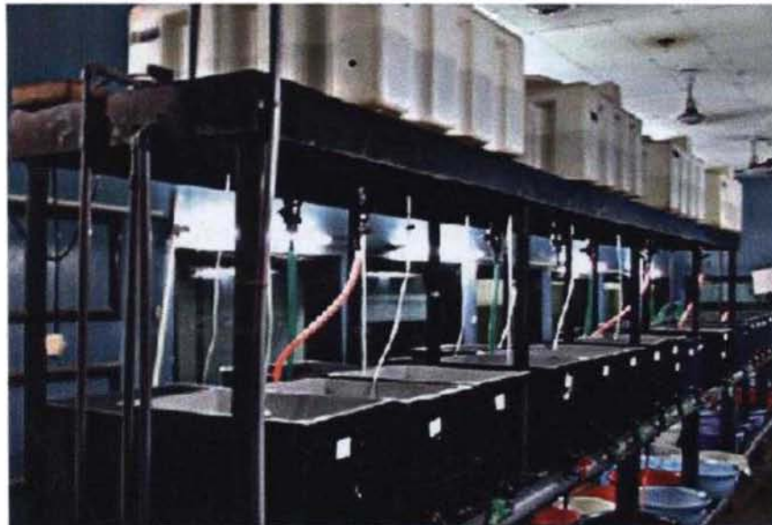
Figure 2.2: Bioassay system used for feeding experiment with P.monodon post larvae for testing antiviral property of marine actinomycetes
