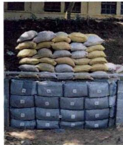
Fig. 5.2 Model gabion box with geotextile lining
