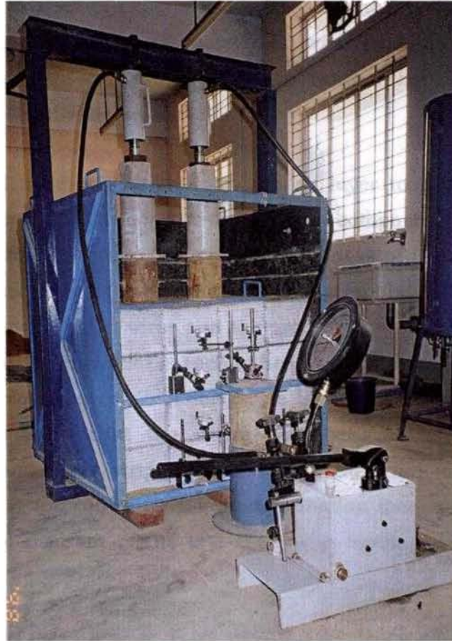
Fig. 5.7 Experimental set up for the model gabion wall
