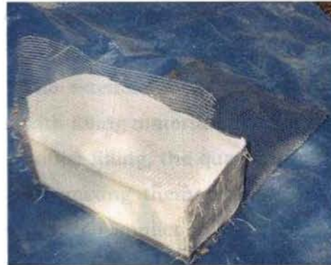
Fig. 5.2 Model gabion box with geotextile lining
