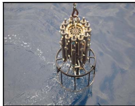
Fig.3.4. Sea-Bird CTD (Underwater unit)
