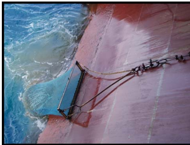
Fig.3.11. Naturalist's Dredge with sample
