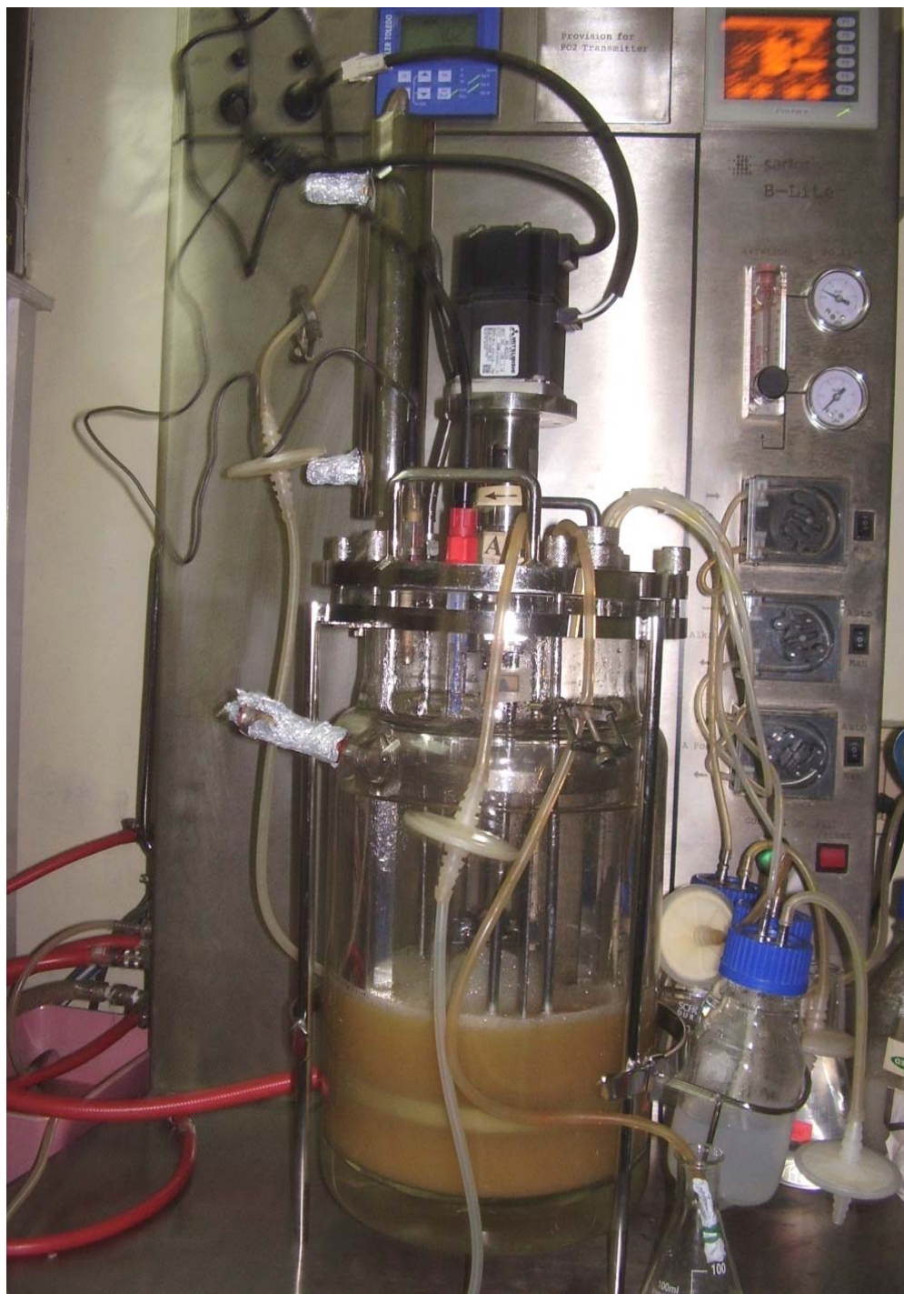
Fig.4.5 Alkaline protease production by Vibrio sp. (V26) in 5 L stirred-tank fermenter
