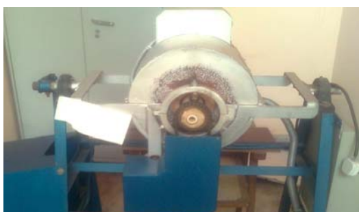
Figure 2.1: Rocking and rotating furnace used for the preparation of ChG glasses.
