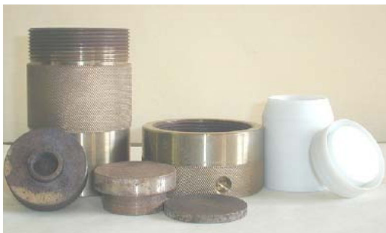
Figure 2.1. General purpose autoclave fabricated for hydrothermal synthesis.
