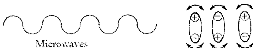
Figure 1: Microwave induced dipole rotation
