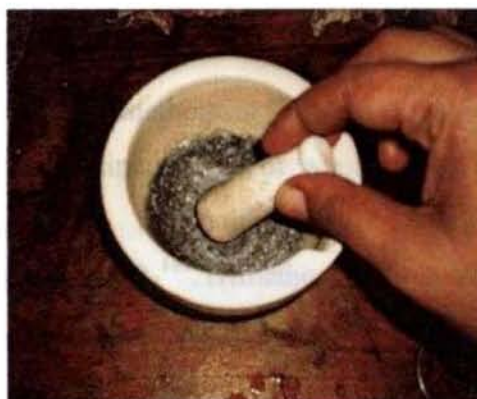
Figure 2.2 Stages involved in the fabrication of a carbon paste sensor.
