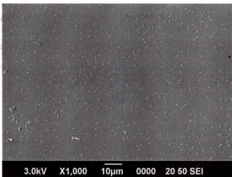
Figure 8.5 SEM image of the polymeric membrane of LO M8 sensor
