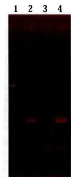
Fig. 4.52 An ethidium bromide stained 1% agarose gel showing the insert amplified with specific primer. Lane 1, Lamda DNA/ EcoRI-Hind III Double Digest marker. Lane 2, amplicon. Lane 3, -ve control (blue colony). Lane 4, amplified plasmid.
