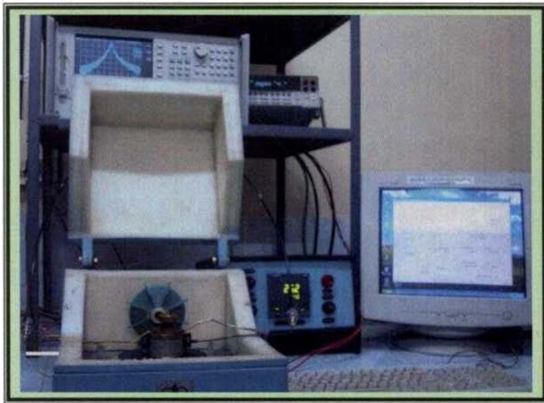
Fig.2.9 Experimental set up used in our lab to measure the microwave dielectric properties
