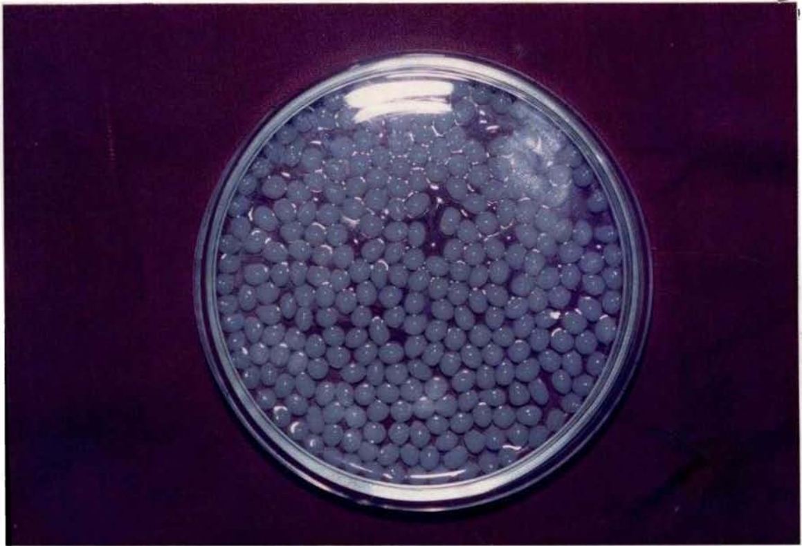
Fig. B.23 : Calcium Alginate Beads used for the Entrapment of T. inflatum
