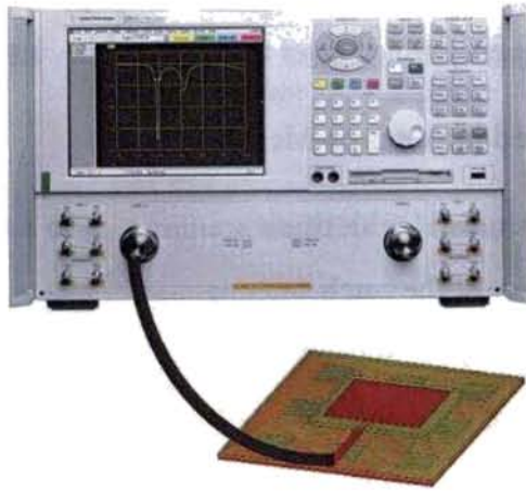
Figure 3.11.1 Measurement set up for Resonant Frequency and Bandwidth
