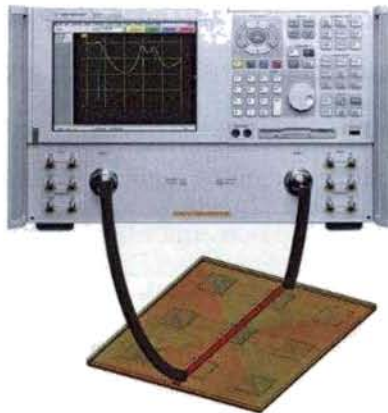
Figure 3.6.1. Measurement setup for reflection and transmission studies
