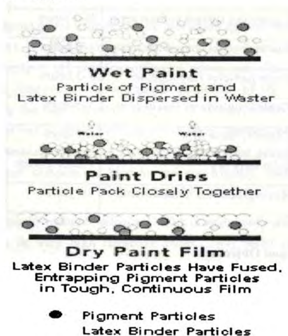
Figure 1.4: Drying mechanism of paint film
