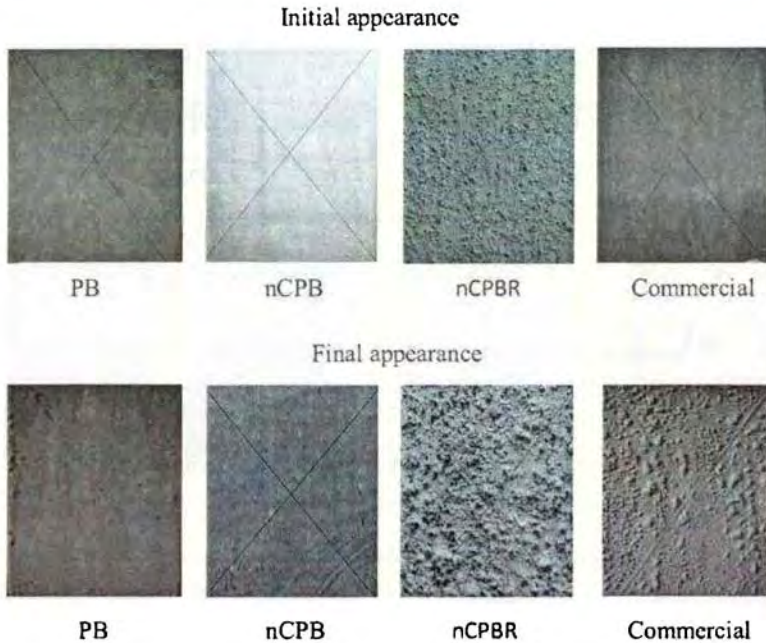
Figure 6c.8: Appearance of specimens before and after salt spray test
