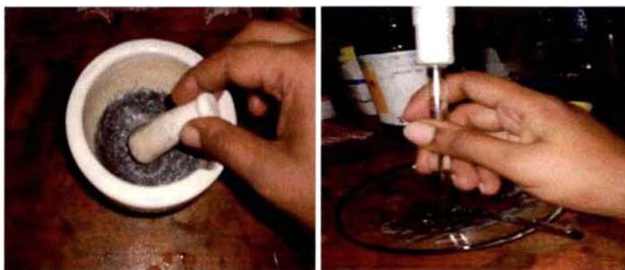
Figure 2.2 Stages involved in the fabrication of chemically modified carbon paste sensor
