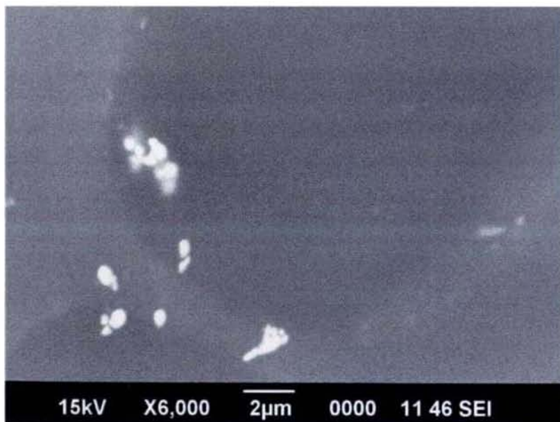
Figure 3.4 SEM image of the polymeric membrane of N 6 sensor
