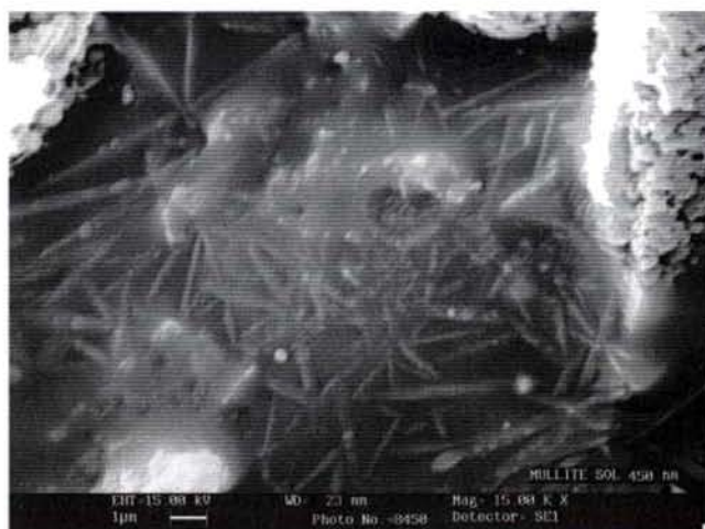
Figure 24. SEM micrograph of mullite coated SiC disc fired at 1300 °C.
