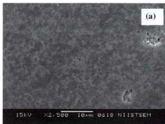
Microstructure of the ground portion were taken and presented in Figure 11. The ground surface micrograph of \text{Al}_2\text{O}_3 -30 \text{LaPO}_4 composite
