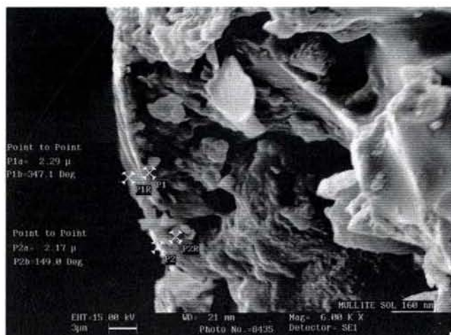
Figure 24. SEM micrograph of mullite coated SiC disc fired at 1300 °C.
