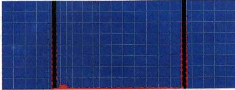
Fig. 6.3 Surface current distribution obtained on the offset fed coplanar waveguide structure with wide centre strip width, dimensions l=9 mm, w=12.5 mm, g=0.5 mm and c=5 mm printed on an FR4 substrate of \epsilon_r=4.7 and thickness h=1.6 mm.
