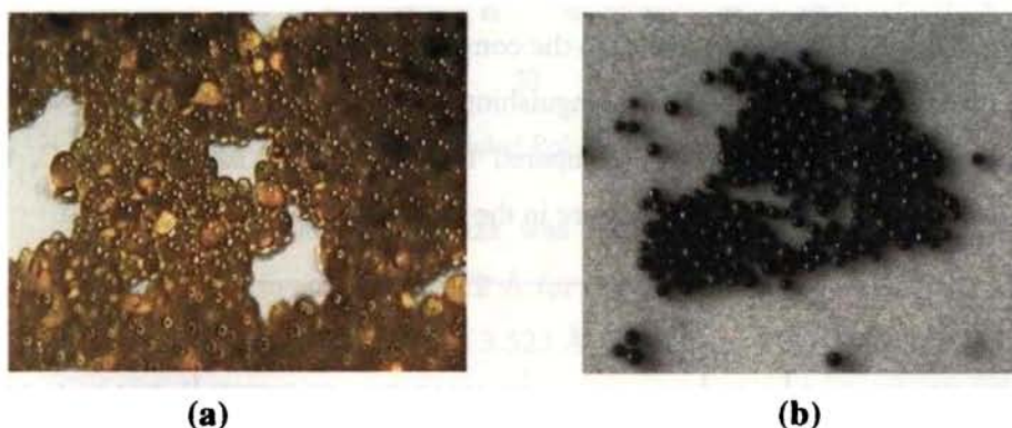
Figure 6.4 Photographs of (a) Polystyrene beads (SAC) (b) SAC-Ni nanocomposites
