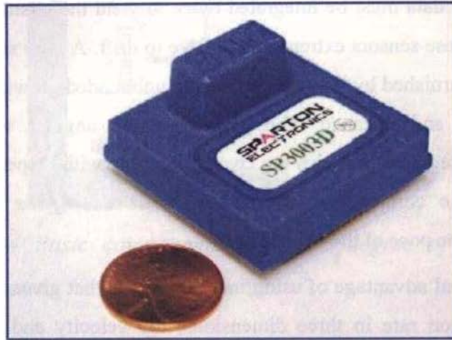
Figure 2.3 A commercially available Electronic Compass SP3003D from Sparton Electronics (2008).
