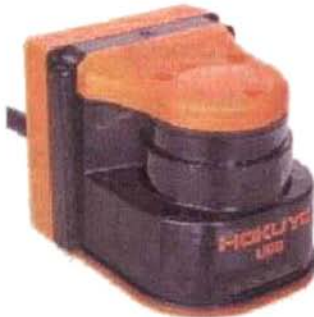
Figure 2.17 UBG-05LN laser scanner from Hokuyo Automatic Company.
