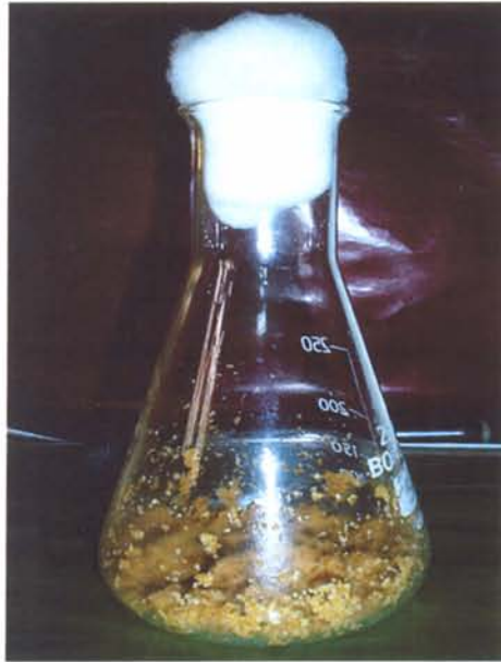
A. SSF set up in a conical flask
