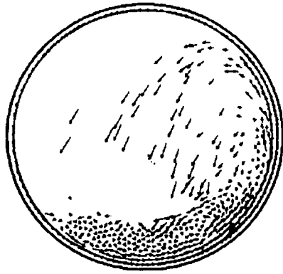
Figure 4.15 (c): Vector plot of centrifuging motion after 3 rotations
