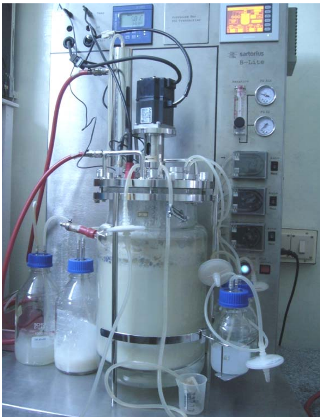
Fig 6.6 Biomass production of Candida S27 in a fermenter using Barnett and Ingram's Modified medium
