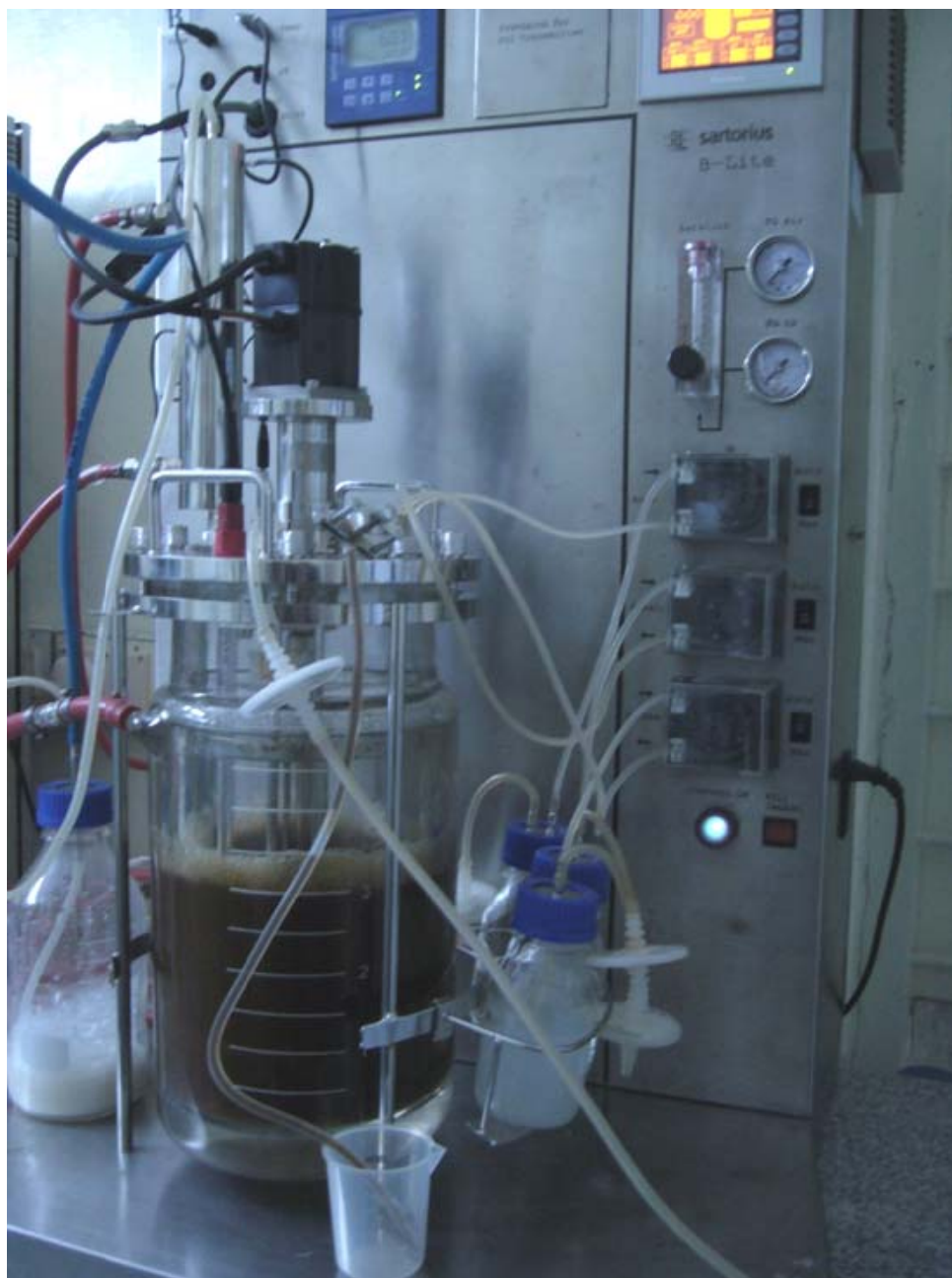
Fig 6.8 Biomass production of Candida sp.S27 in a fermenter using Molasses-Yeast extract medium
