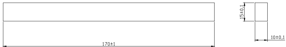
Fig 3.4 Specimen for Determination of Poisson's ratio
