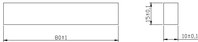
Fig 3.3 Specimen for Out of plane Shear Test
