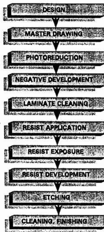
FIGURE 3.1 Step-by-step procedure of photolithographic technique
