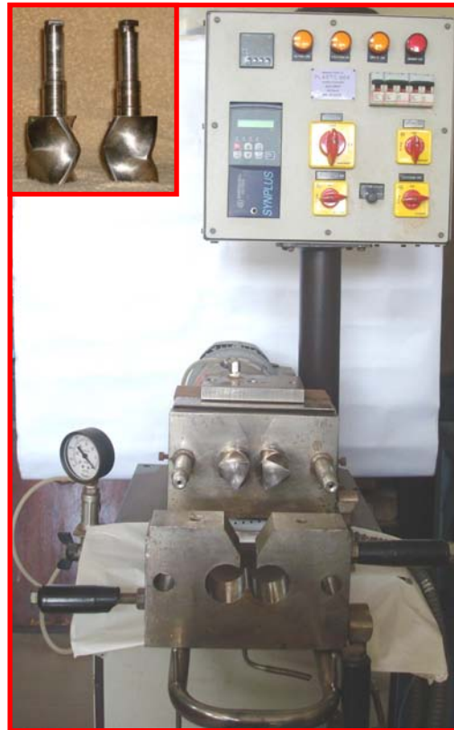
Fig. 2.3 Kneading machine used in melt mixing technique. Inset figure shows the sigma blades.
