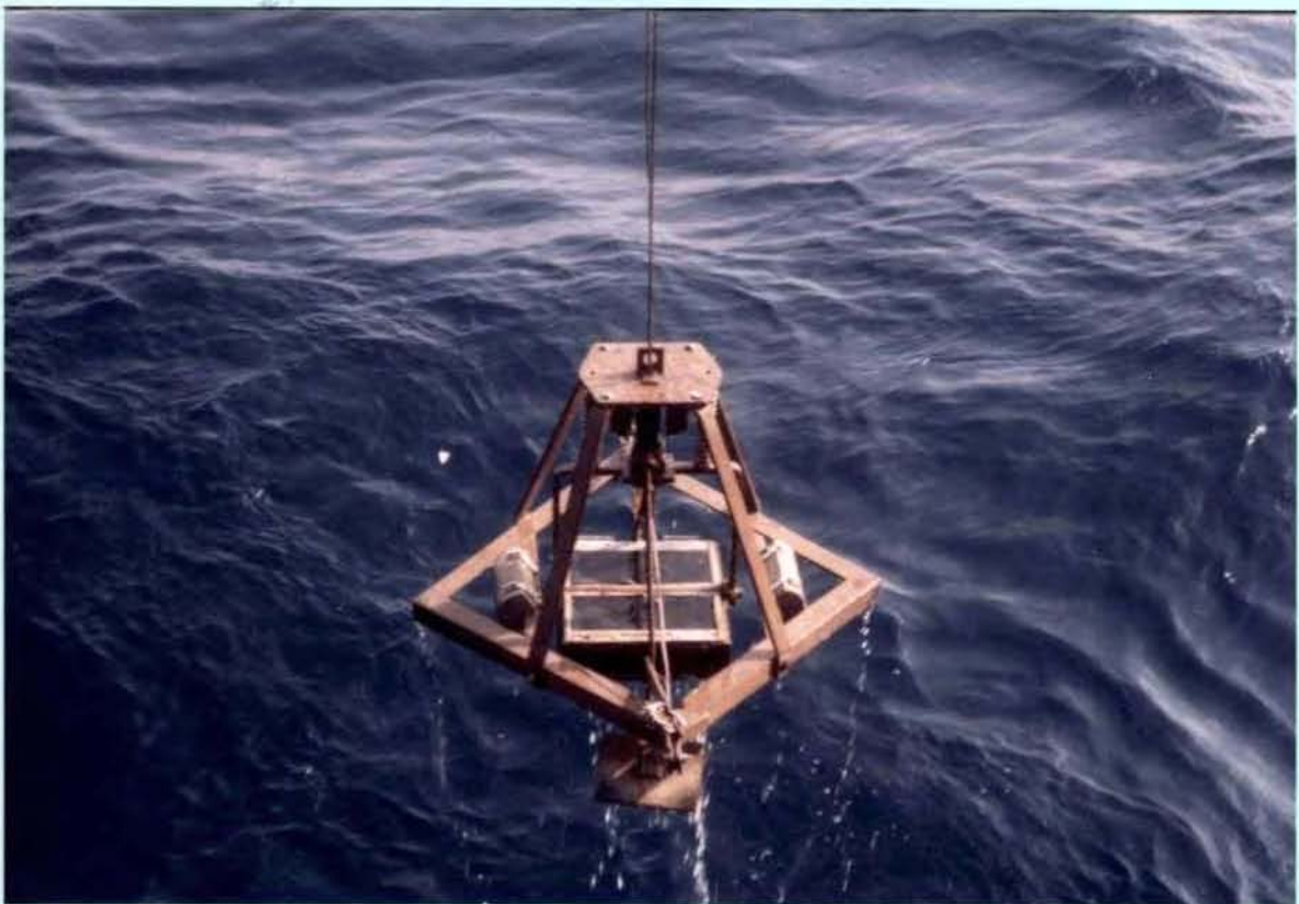
3B. Smith-Mc Intyre grab: during hauling up
