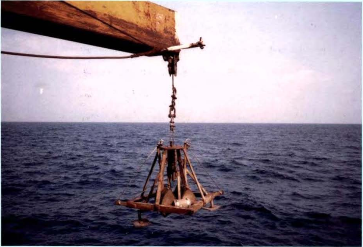
3A. Smith-Mc Intyre grab: ready to deploy
