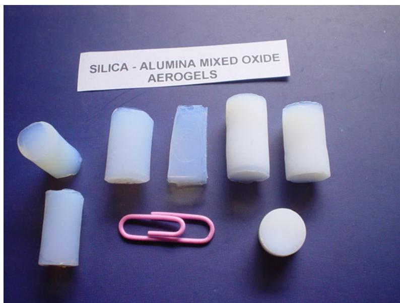
**Fig. 2.2.2.** Photograph of silica-alumina mixed oxide aerogels
