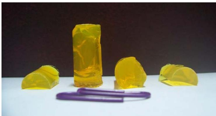
**Fig. 4.1. 15.** Photograph of Silica-Titania aerogel prepared by impregnation
