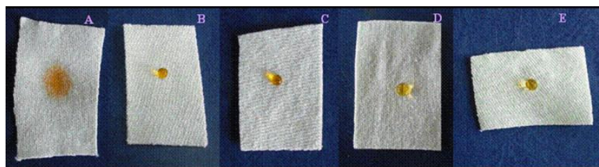
Fig. 4.2.11. Photographs of water drops on coated textiles prepared by changing the concentration of MTMS in the coating solution A) 0.05 B) 0.5 C) 1 D) 2.5 E) 9
