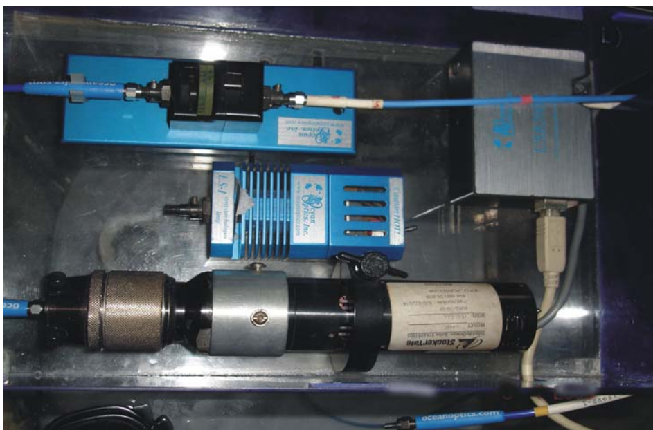
Fig. 3.6 Top view of the portable LIFRS developed for clinical studies of dental caries, with diode laser at the bottom, spectrometer to the left, in-line filter holder at top and tungsten halogen lamp aligned at centre of an acrylic box of dimensions 12 x 8 x 3 inches.
