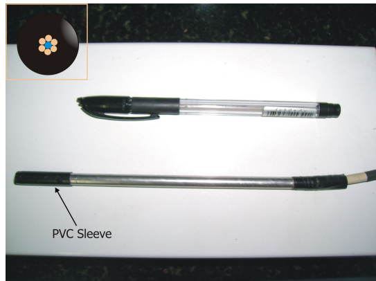
Fig. 3.2 Stainless extreme of the reflection measuring probe inserted with PVC sleeve. In subset 6-around-1 close geometry to ensure the highest fluorescence yield, optimized overlapping of excitation and emission areas, of the reflection probe is exhibited.
