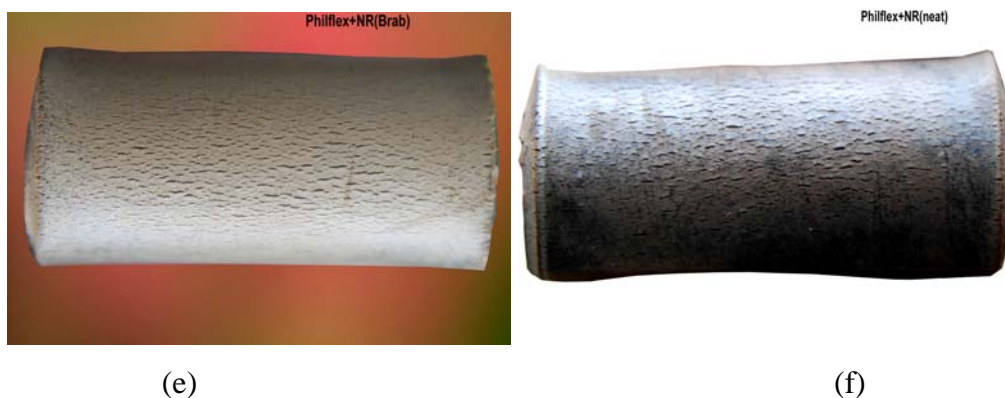
Figure 7.6 (a-f): The photographs of ozone cracked surface of NR vulcanizates after 7 hours
