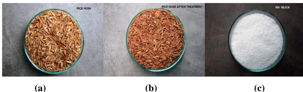
Figure 8.6 (a) rice husk (b) rice husk after treatment with acid (c) RHsilica
