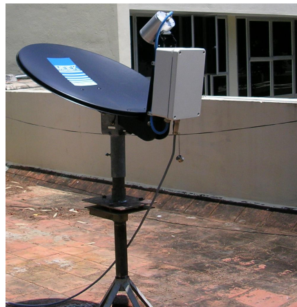
Figure 2.6. Micro Rain Radar (MRR) deployed in the premises of our institute, Centre for Earth Science Studies (CESS), Thiruvananthapuram.
