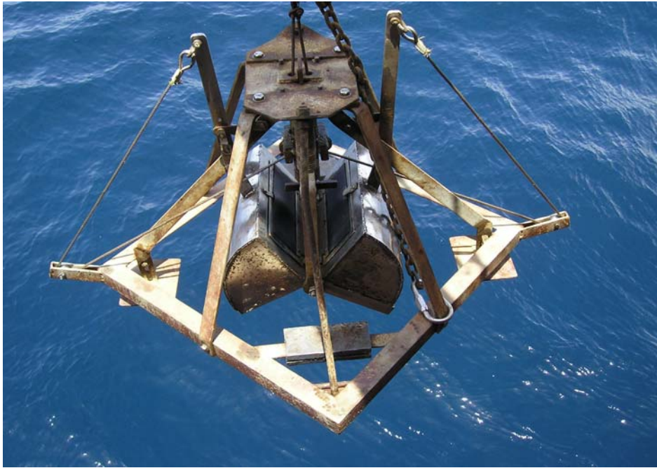
Fig. 2.6 Smith McIntyre Grab used for sediment sample collection
