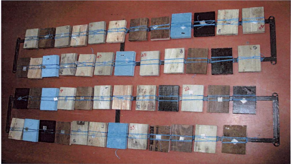
Fig. 3.18: Panels arranged and kept ready on iron rack for immersion in the estuary
