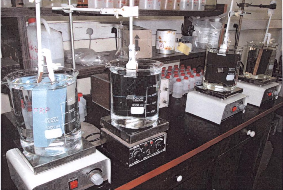
Fig. 6.7: Experimental set up of studies for control of leaching in the accelerated condition
