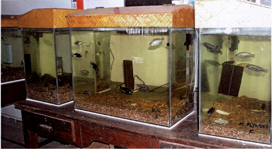
Fig. 3.17: Laboratory set up of stagnant leaching studies
