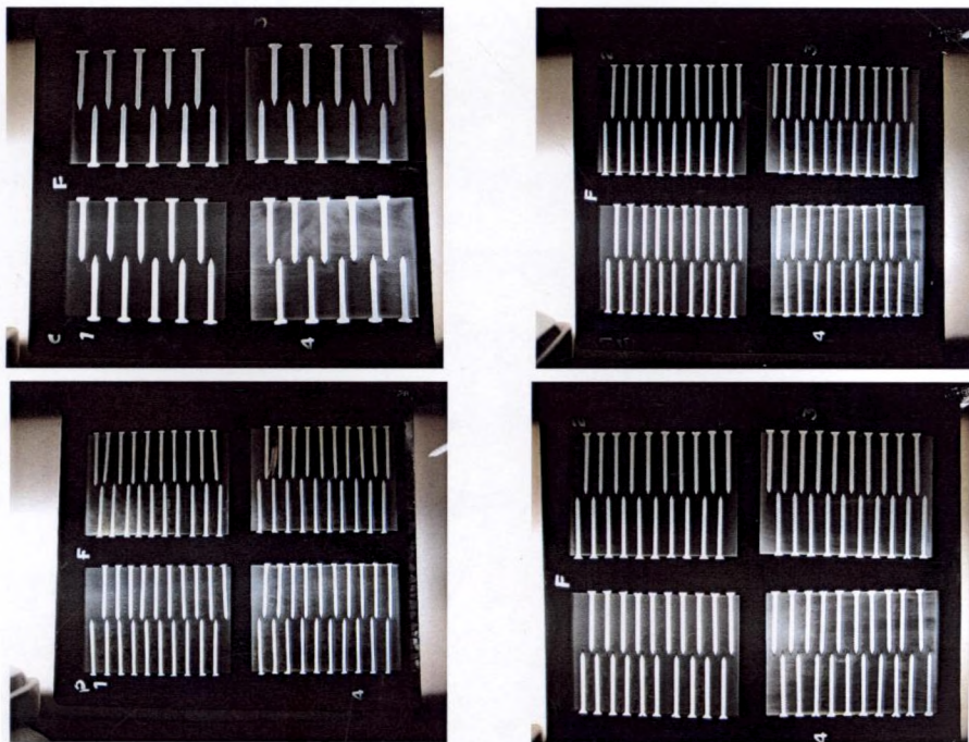
Fig. 7.12: X-ray photographs of CCA treated rubber wood panels of untreated and of three different retentions nailed with copper, iron, painted iron and galvanized iron nails after exposure in the estuary
