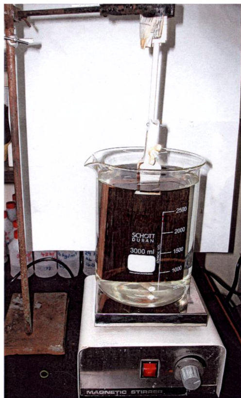
Fig. 3.17: Laboratory experimental set up of accelerated leaching studies
