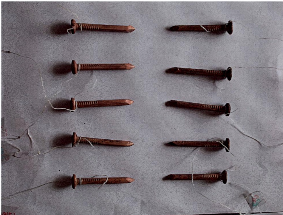
Fig. 7.8: Copper nails removed from the wood panel exposed in the estuary
