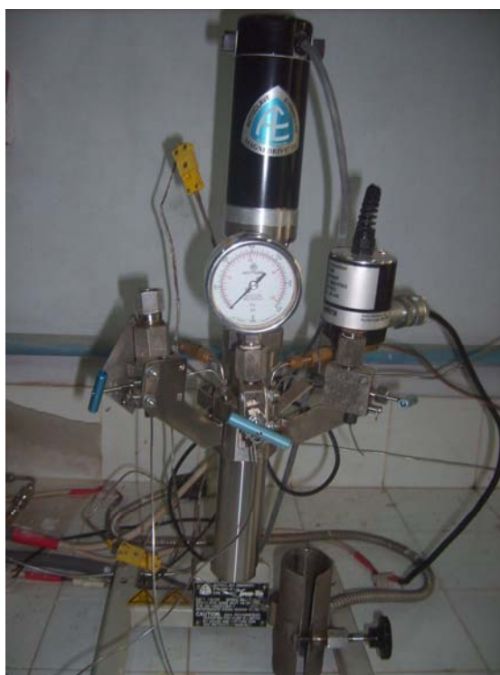
Figure 1: Bench top mini-reactor (100 mL)
