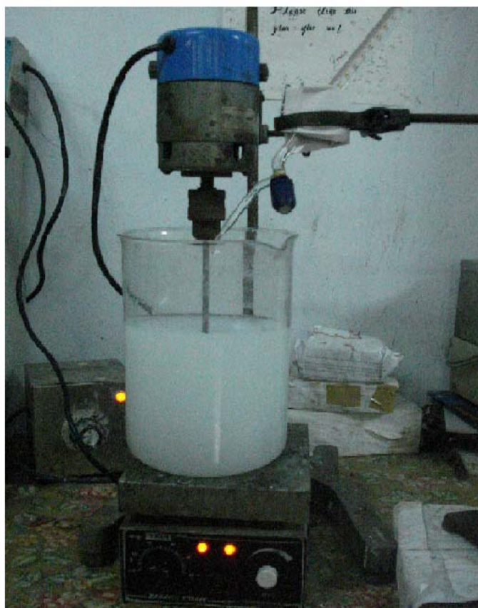
Figure 2.1. Reactor with stirring cum heating arrangement
