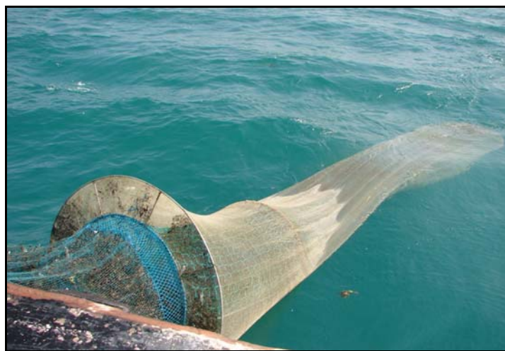
Fig 2.2 Radial Escapement Device-150 mm modified for reducing masking effect of the cover
