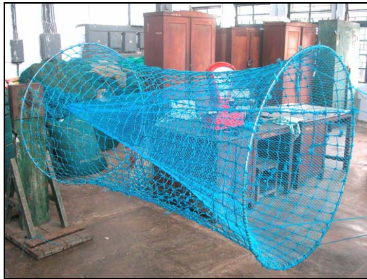
Fig 2.1 Radial Escapement Device with 150 mm square mesh escapement section
