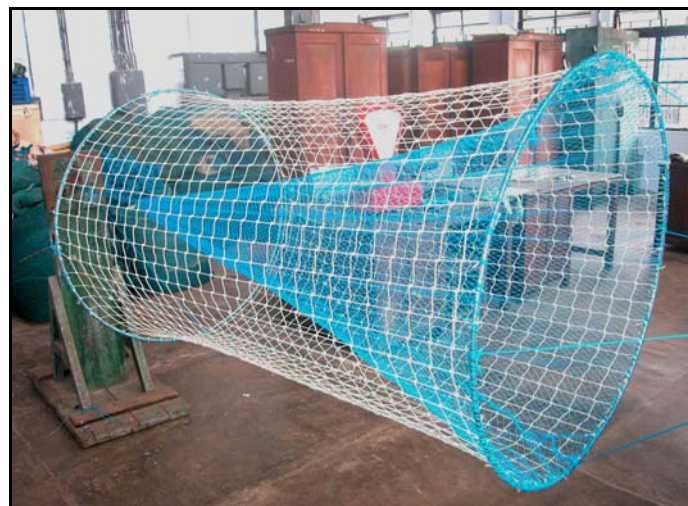
Fig 2.3 Radial Escapement Device with 100 mm square mesh escapement section
