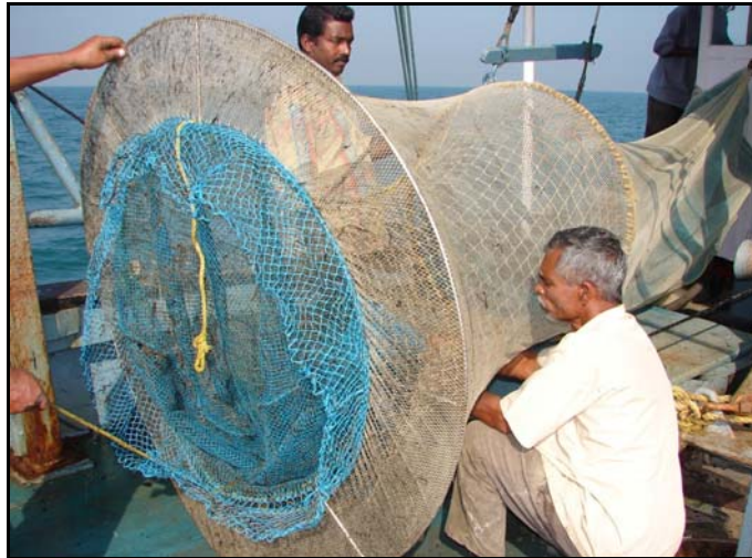
Fig 2.4 Radial Escapement Device-100 mm modified for reducing masking effect of the cover
