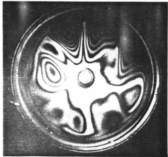
Fig.2.16 Reconstructed image of a vibrating loud speaker.
