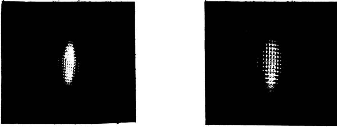
Fig 5.3 Fourier spectrum of a wire mesh formed by a.Glass lens, b.Holographic lens.
