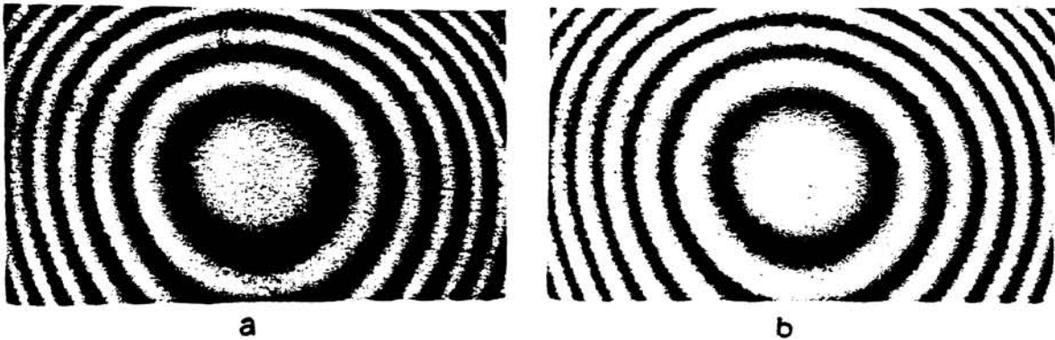
Fig 3.5 Fringes obtained a. In object beam direction b. Reference beam direction
