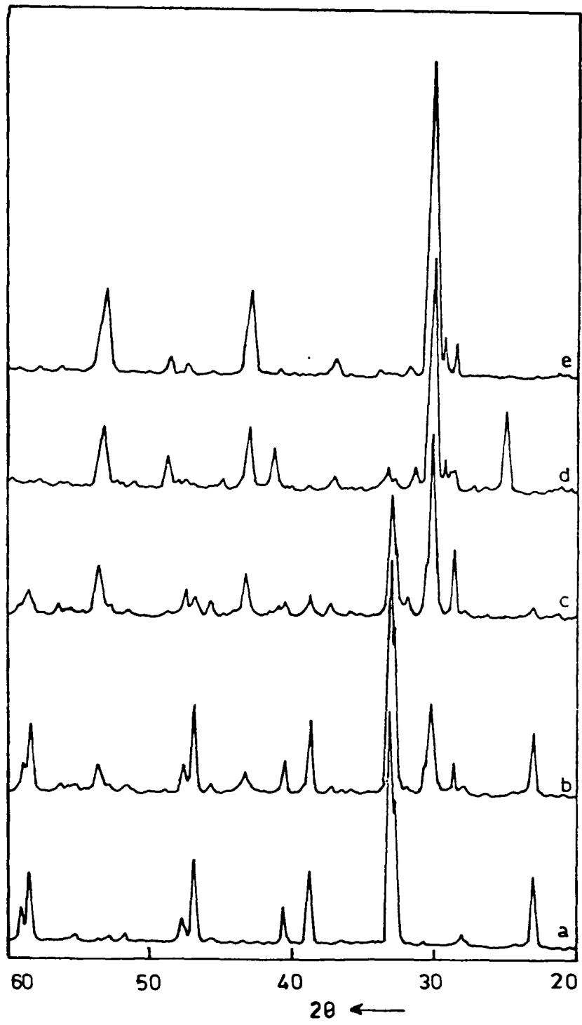
Fig. 5.14: XRD pattern of BYSbO-YBCO composites for different vol % of BYSbO (a) 0, (b) 30, (c) 50, (d) 70, (e) 100
