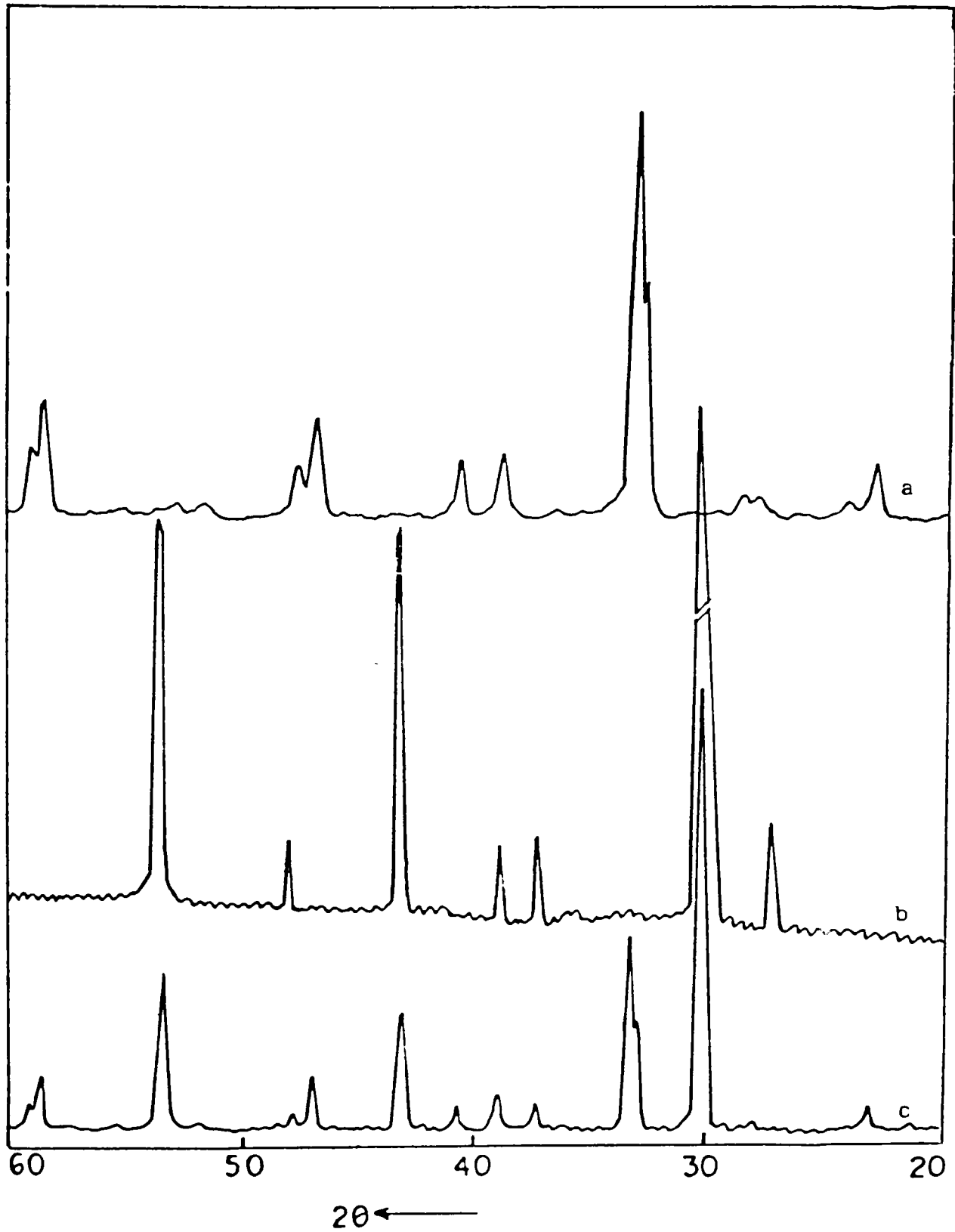
Fig. 4.20: XRD pattern of (a) pure YBCO, (b) pure BYSbO, (c) 1:1 mole mixture of YBCO:BYsbo heated at 950^\circ\text{C} for 10 hrs.
