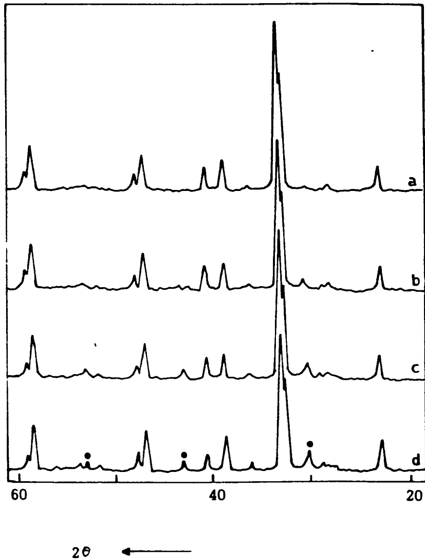
Fig. 3.10: XRD pattern of different wt % of \text{Sb}_2\text{O}_3 added YBCO cooled slowly to room temperature in oxygen atmosphere
