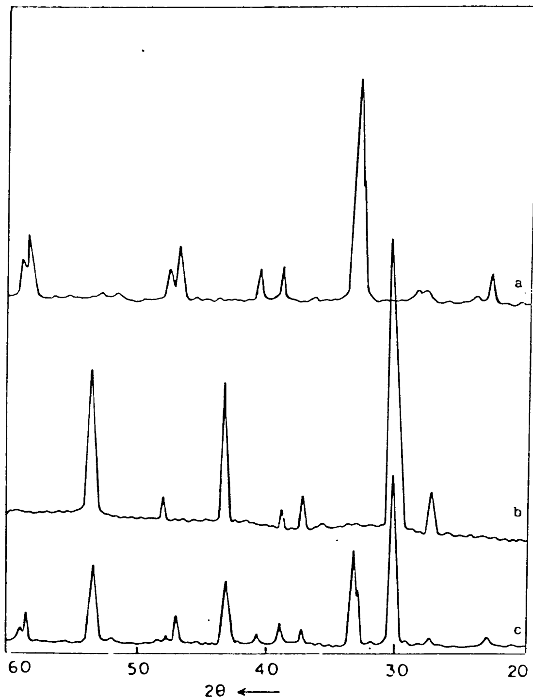
Fig. 4.16: XRD pattern of (a) pure YBCO, (b) pure BYZO, (c) 1:1 mole mixture of YBCO : BYZO heated at 950°C for 10 hrs.
