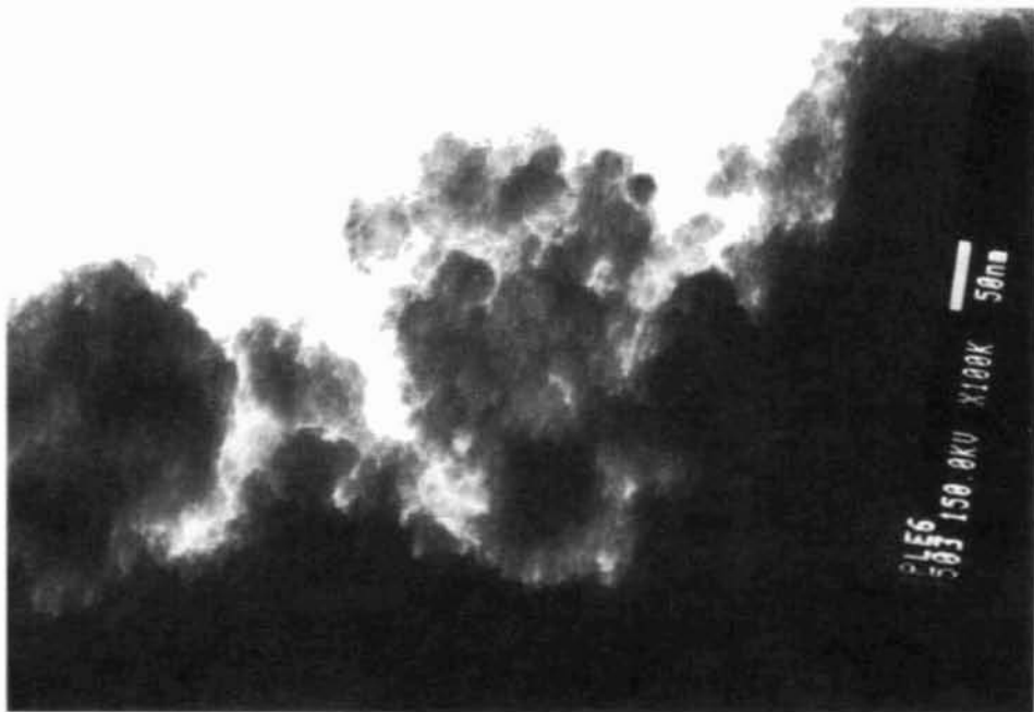
Figure 3.7 Transmission electron micrograph for 10 hours dry milled zinc ferrite.
