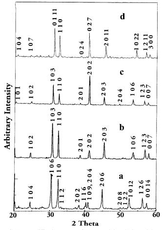
FIG. 1. X-ray diffraction patterns of (a)  $BaLa_4Ti_4O_{15}$ , (b)  $SrLa_4Ti_4O_{15}$ , (c)  $CaLa_4Ti_4O_{15}$ , and (d)  $Ca_2La_4Ti_5O_{18}$ .
