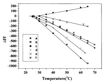
FIG. 4. Plot of  $\Delta f/f$  against temperature (a) SrLa<sub>4</sub>Ti<sub>4</sub>O<sub>15</sub>, (b) CaLa<sub>4</sub>Ti<sub>4</sub>O<sub>15</sub>, (c) Ca<sub>2</sub>La<sub>4</sub>Ti<sub>5</sub>O<sub>18</sub>, (d) Ca<sub>2</sub>La<sub>4</sub>Ti<sub>5</sub>O<sub>17</sub>, and (e) CaLa<sub>8</sub>Ti<sub>9</sub>O<sub>31</sub>.
