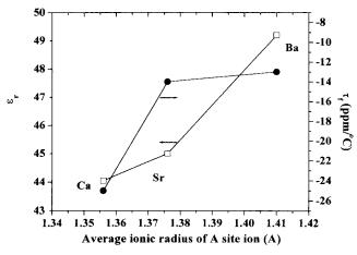
FIG. 5. Variation of  $\epsilon_r$  and  $\tau_f$  with average ionic radius of A site ion for MLa<sub>4</sub>Ti<sub>4</sub>O<sub>15</sub>.
