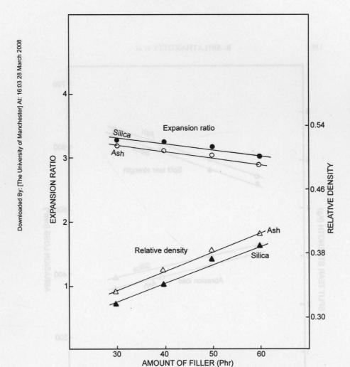
FIGURE 1 Variation of expansion ratio and relative density with increase in filler loading.
