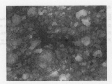
FIGURE 6 Optical photograph of the compound containing 40 Phr white ash in NBR/PVC based MC sole compound.
