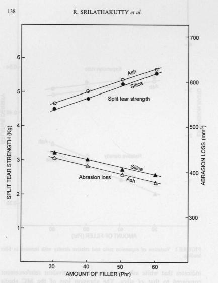
FIGURE 2 Variation of split tear strength and abrasion loss with increase in filler loading.
