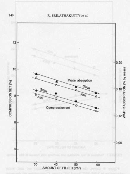
FIGURE 4 Variation of compression set and water absorption with increase in filler loading.
