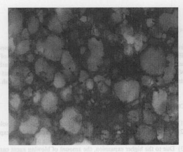
FIGURE 5 Optical photograph of the compound containing 40 Phr silica in NBR/PVC based MC sole compound.
