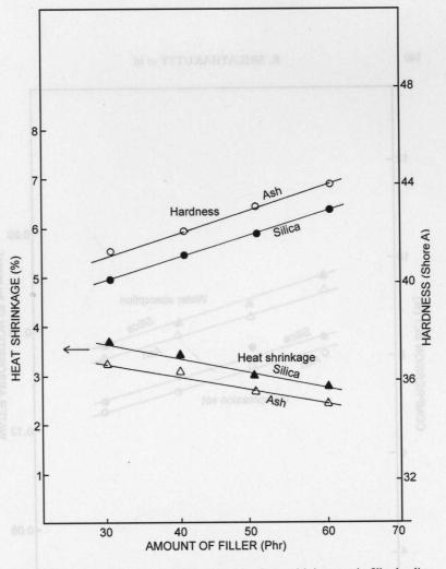
FIGURE 3 Variation of heat shrinkage and hardness with increase in filler loading.
