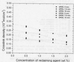
Figure 31 Crosslink density as a function of concentration
