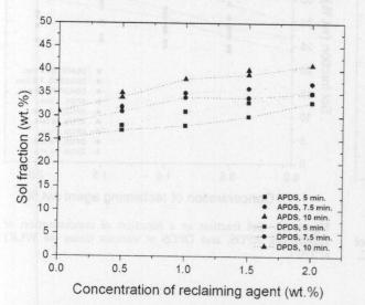
Figure 13 Sol fraction as a function of concentration of APDS and DPDS at various times for WLP1 at 1986
