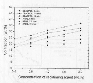
**Figure 9** Sol fraction as a function of concentration of DBADPDS and APDS at various times for WLR1 at 160°C.
