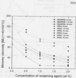
Figure 22 Mooney viscosity as a function of concentration of DBADPDS, APDS, and DPDS at various times for WLR2 at 170°C
