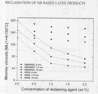
Figure 20 Mooney viscosity as a function of concentration of DBADPDS and APDS at various times for WLR2 at 150°C.
