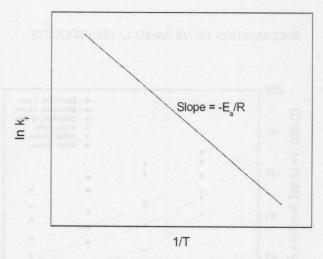
**Figure 2** The Arrhenius plot of  $\ln k_r$  versus 1/T.
