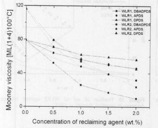
Figure 37 Mooney viscosity of WLR1 and WLR2 as a function of concentration of the realizing agent at 170°C
