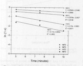
Figure 44 Determination of rate constant for WLR1 with APDS at different temperatures.
