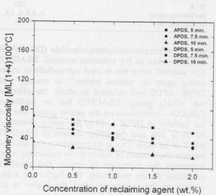
**Figure 6** Mooney viscosity as a function of concentration of APDS and DPDS at various times for WLR1 at 180°C.
