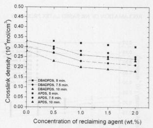
**Figure 10** Crosslink density as a function of concentration of DBADPDS and APDS at various times for WLR1 at 160°C.
