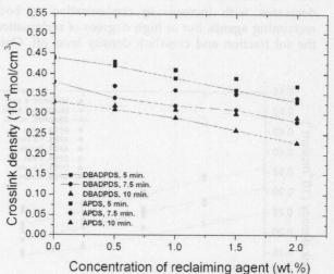
**Figure 27** Crosslink density as a function of concentration of DBADPDS and APDS at various times for WLR2 at 160°C.
