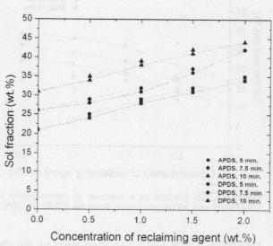
**Figure 30** Sol fraction as a function of concentration of APDS and DPDS at various times for WLR2 at 180°C.
