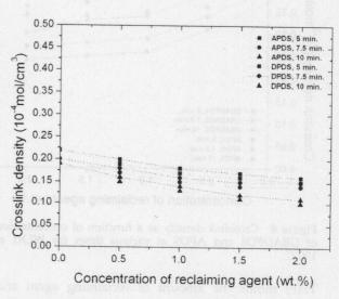
**Figure 14** Crosslink density as a function of concentration of APDS and DPDS at various times for WLR1 at 180°C.
