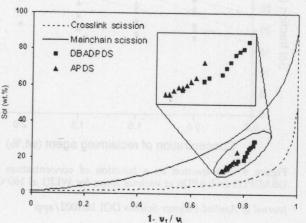
Figure 15 Fraction of sol of WLR1 against relative
