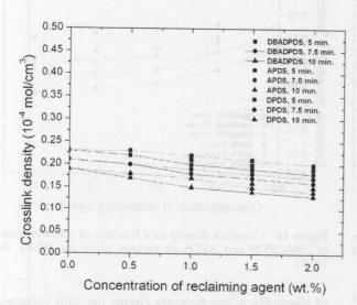
**Figure 12** Crosslink density as a function of concentration of DBADPDS, APDS, and DPDS at various times for WLR1 at 170°C.
