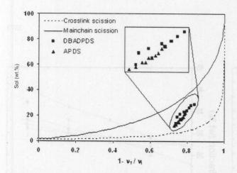
Figure 32 Fraction of sol of WLR2 against relative decrease in crosslink density at 150°C.
