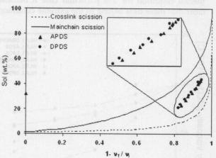
Figure 35 Fraction of sol of WLR2 against relative decrease in crosslink density at 180°C.
