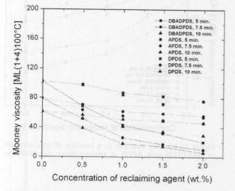
**Figure 5** Mooney viscosity as a function of concentration of DBADPDS, APDS and DPDS at various times for WLR1 at 170°C.
