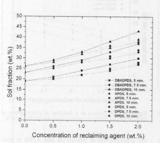
Figure 28 Sol fraction as a function of concentration of DBADPDS, APDS, and DPDS at various times for WLR2 at  $170^{\circ}$ C.
